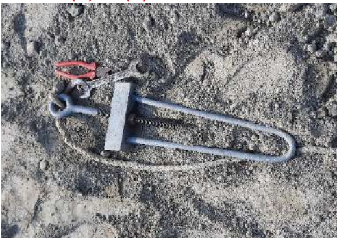
(g) Turnbuckle to tighten wires and ropes
